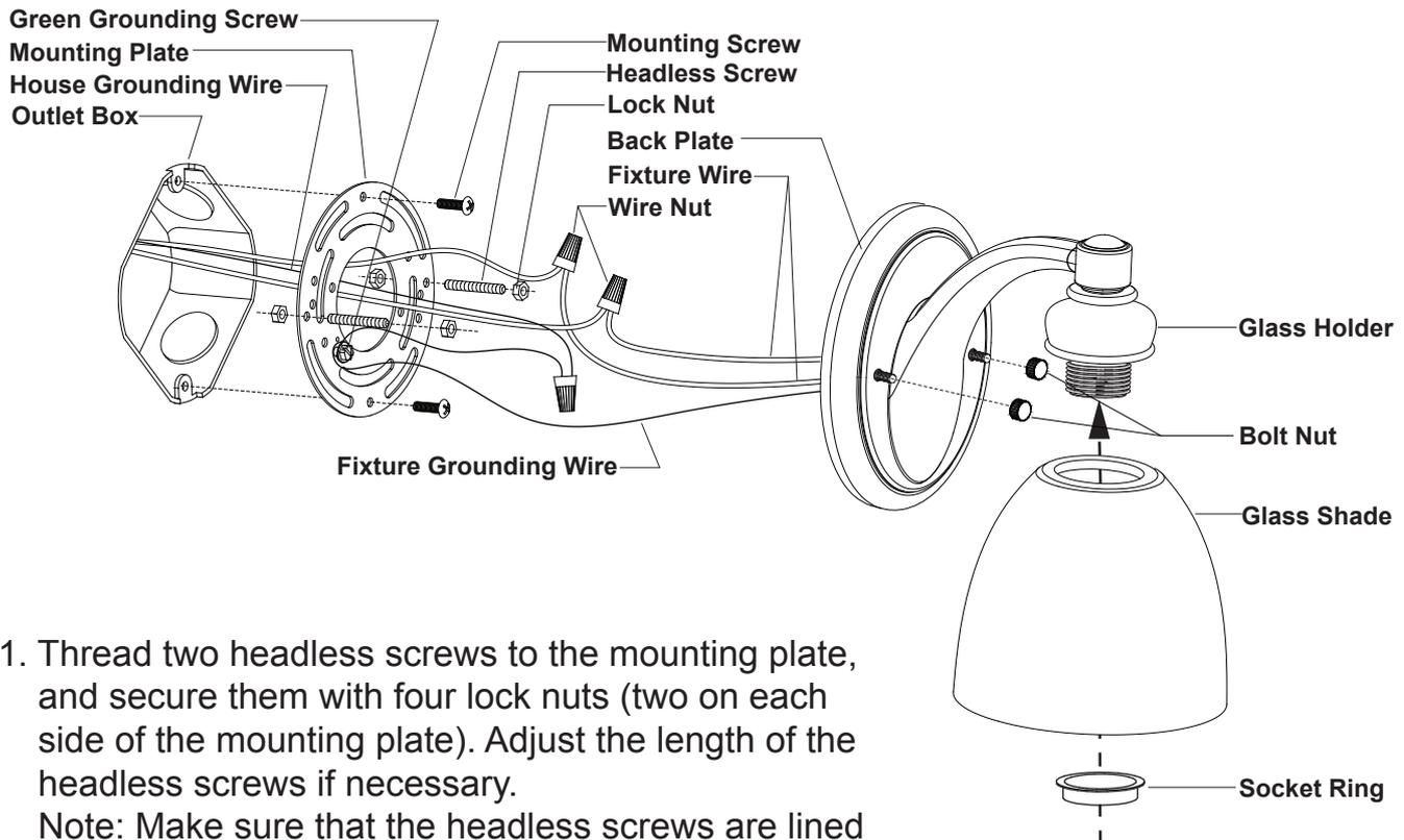
1. Thread two headless screws to the mounting plate, and secure them with four lock nuts (two on each side of the mounting plate). Adjust the length of the headless screws if necessary.
