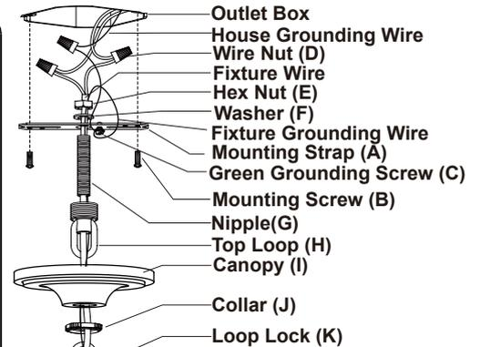
1. Attach nipple to the mounting strap, then secure it with a washer and hex nut.
