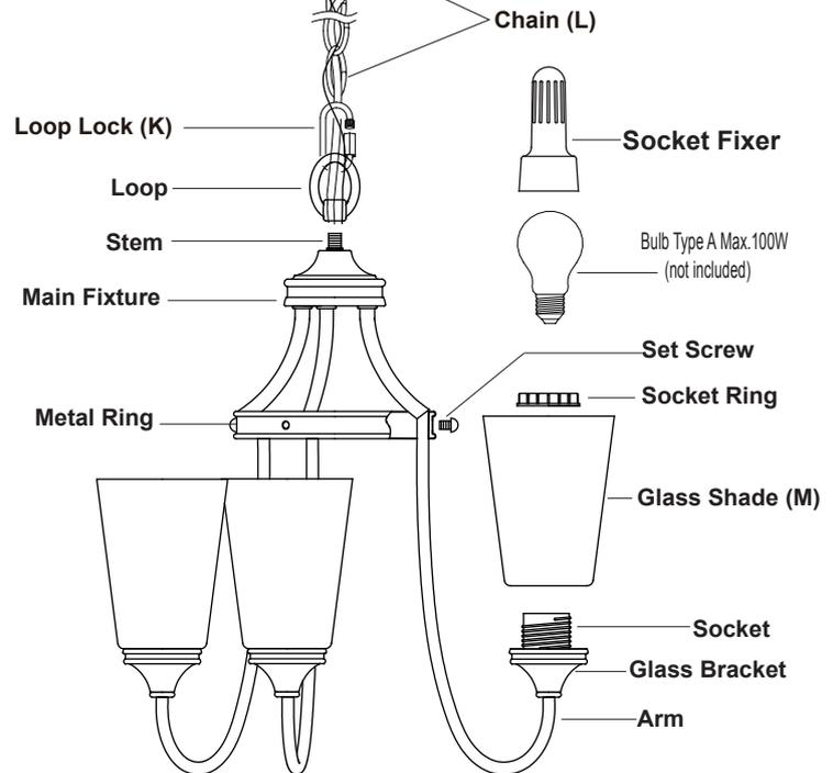
12. Install bulbs(not included). See relamping label at socket area or packaging for maximum allowed wattage.
