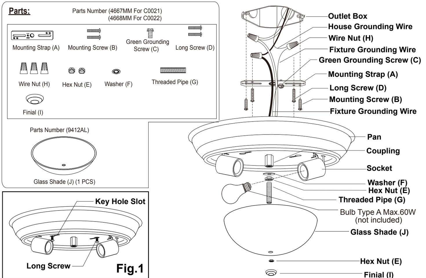
1. Attach the two long screws to the mounting strap, and screw in 2 to 3 turns.
