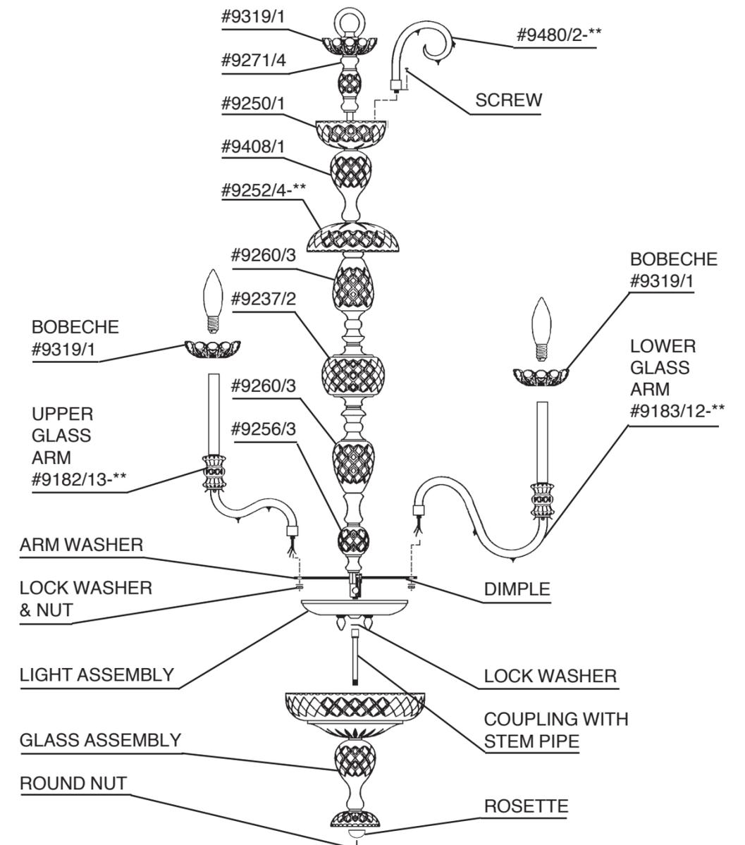
**8** Install scrolls into washer with screws provided. ALTERNATELY install upper and lower arms into the washer. Line up holes in arms with dimple in washer. Use lock washer and nut to secure arms in place.
