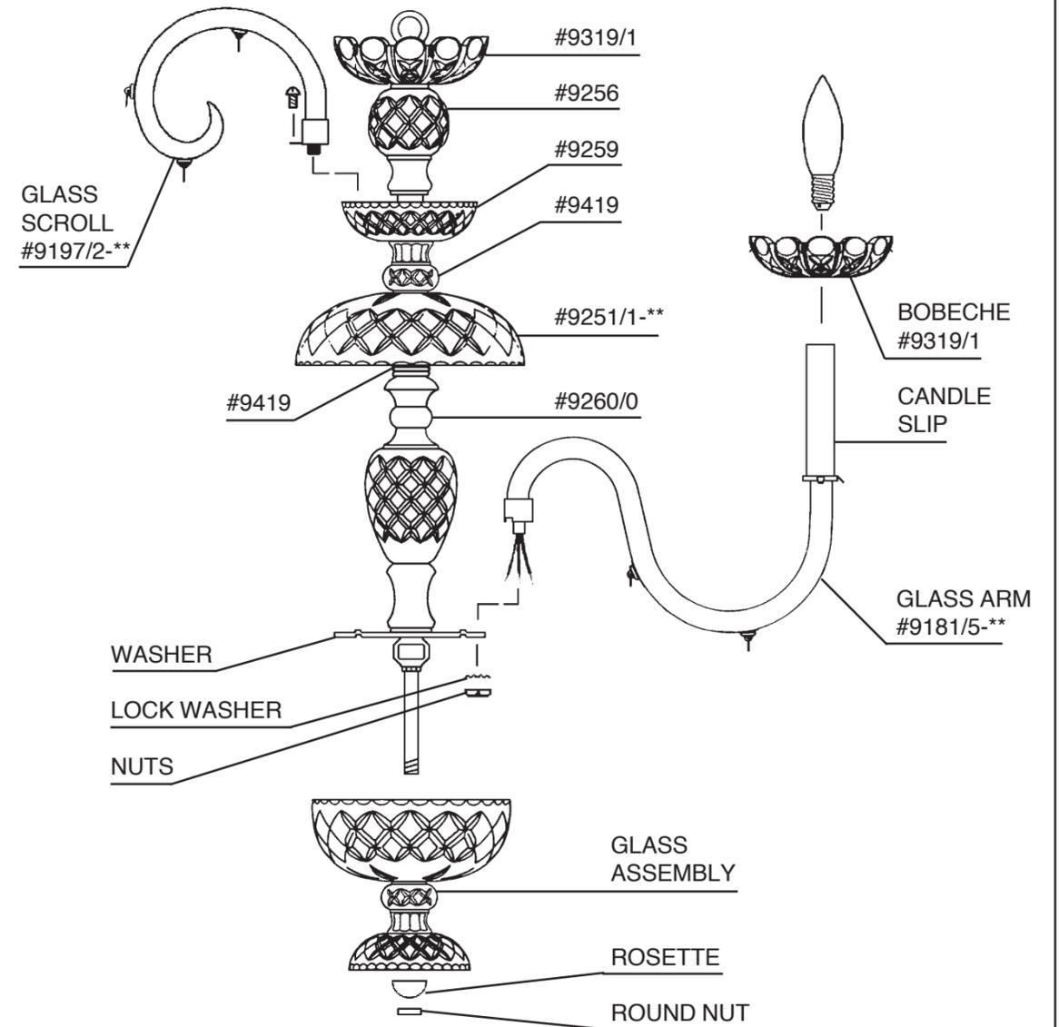
**8** Install scrolls into washer with screws provided. Install arms into large arm washer. Line up holes in arms with dimple in washer. Use lock washer and nut to secure arms in place.
