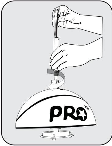
Thread the downrod onto the motor housing making sure the wires don't get twisted.
