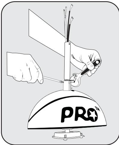
Insert safety bolt (S6) through flange & downrod and attach nut. Tighten firmly.
