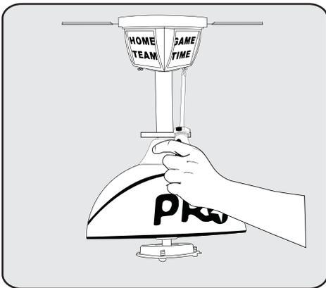
Tighten screws firmly.
