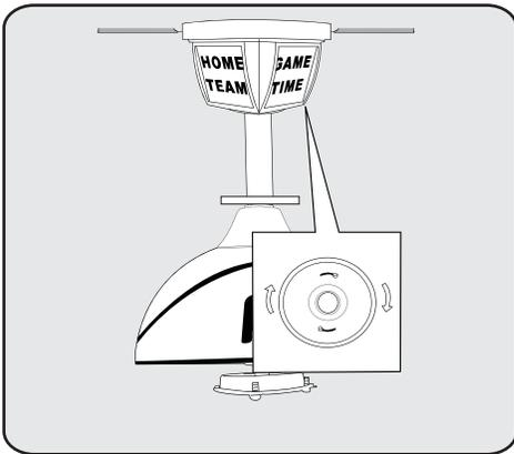
Twist clockwise to lock into place.
