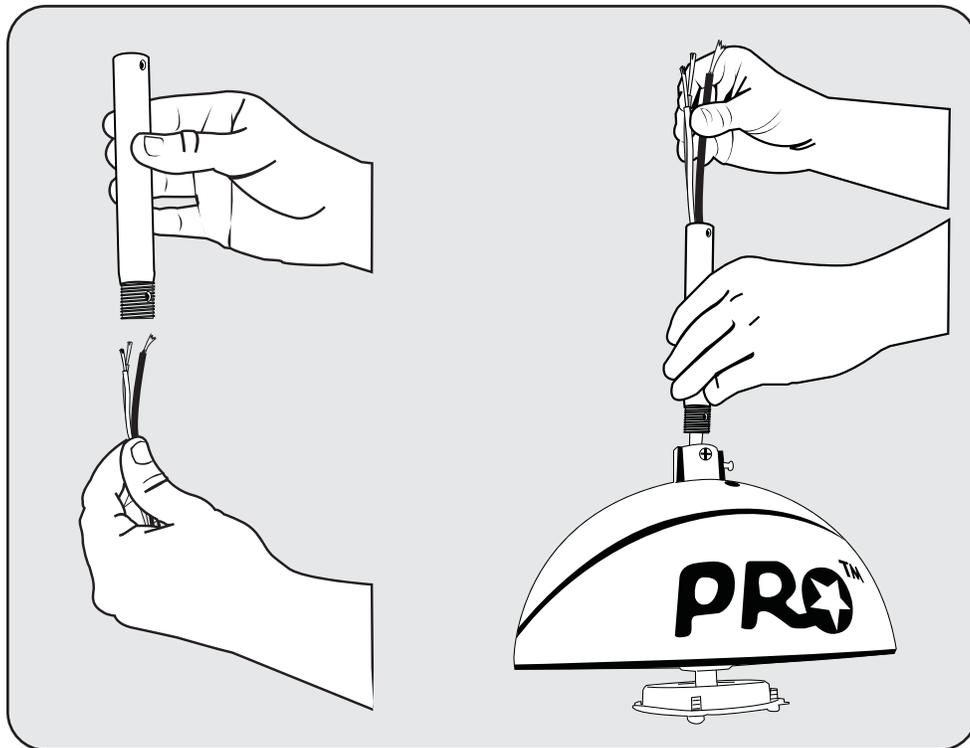
Insert fan wires through downrod.
