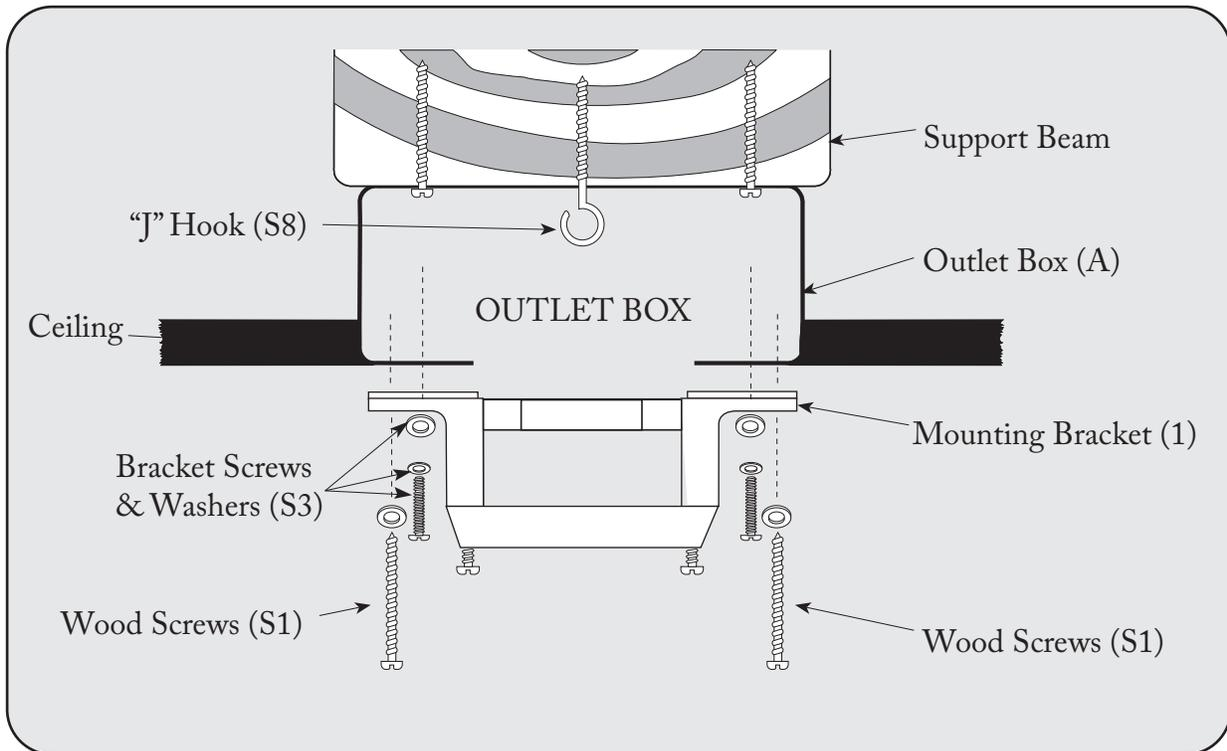
**NOTE:** Do not mount directly to sheet rock or ceiling tile.
