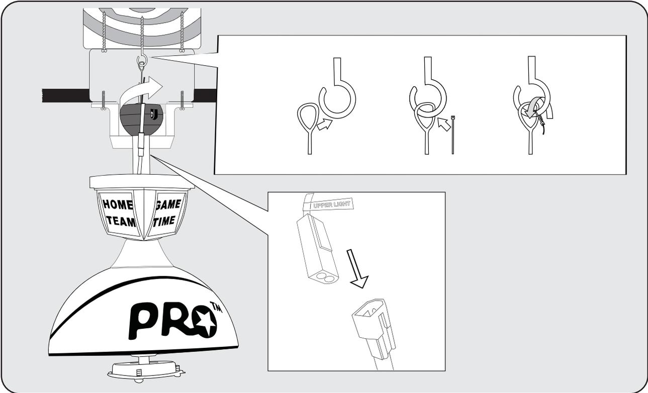
Lift fan onto the mounting bracket (1). Turn housing until hanging ball seats itself into ball socket (listen for click).
