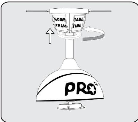
Seat the canopy screw cover into slots and twist to lock.
