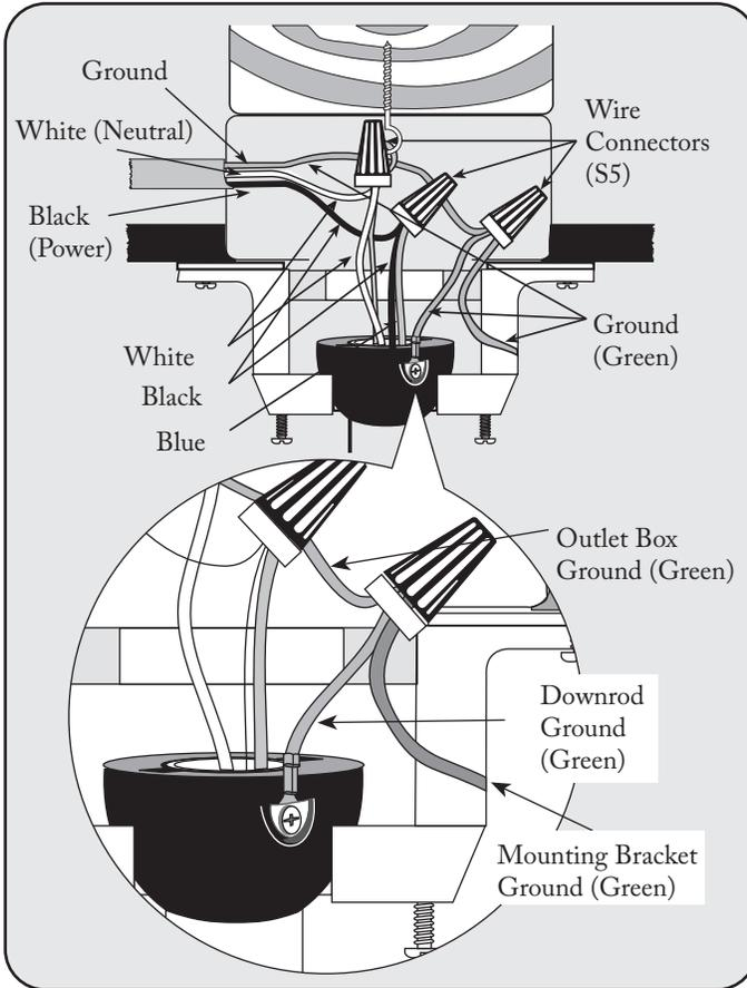
1. Connect fan wires to ceiling wires: white fan wire to white outlet wire, black to black and green to green. Wire connectors (S5) are provided for your convenience. If an additional blue wire is present then also connect the blue wire to the black wire. (Optional light kit may be wired to individual wall switches, if desired.)
